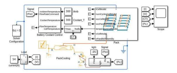
Thermal analysis comparison of a new and aged lithium-ion battery using Simscape Battery.
